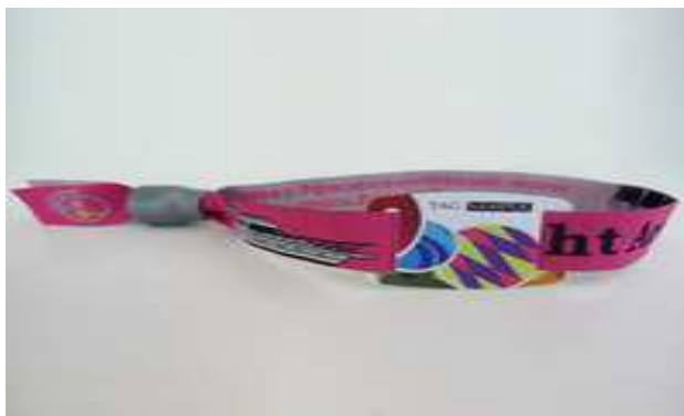
Figure 1. Example of an all-inclusive access control bracelet with non-contact tag.
